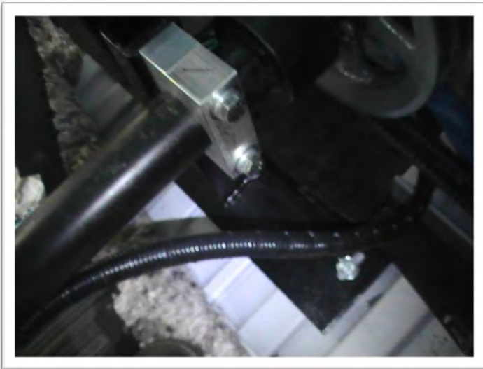
50. When drive shaft, clutch, and lower pulley are aligned, drill and bolt the rear shaft mount in place with two 3/8-16 x 1 3/4:" bolts. **Before drilling through the floor of the van, check for any hazardous obstructions. Verify alignment using a straight edge. Tighten front and rear clamps and re-check alignment.
